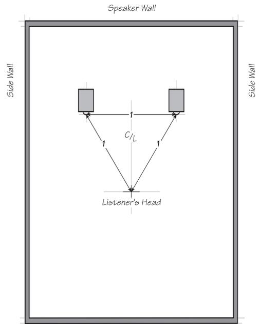
In the near field position the speakers and the listener's head are the points of an equilateral triangle. Near field listening gives the perfect stereo field. It is frequently used in the recording studio to position the microphones and the voice in the mix. The near field listening position is determined by the "center to center" distance of the speakers and the distance to the listener's head. It does not refer to the room in any way.
