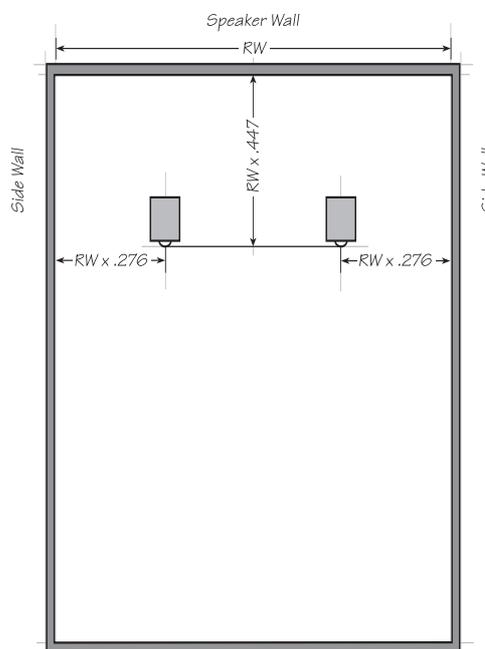
Active nodes are the main concern when placing speakers in a rectangular room. A node, or the frequency where speakers and parallel walls interact, is proportional to the speaker to the wall distance.
