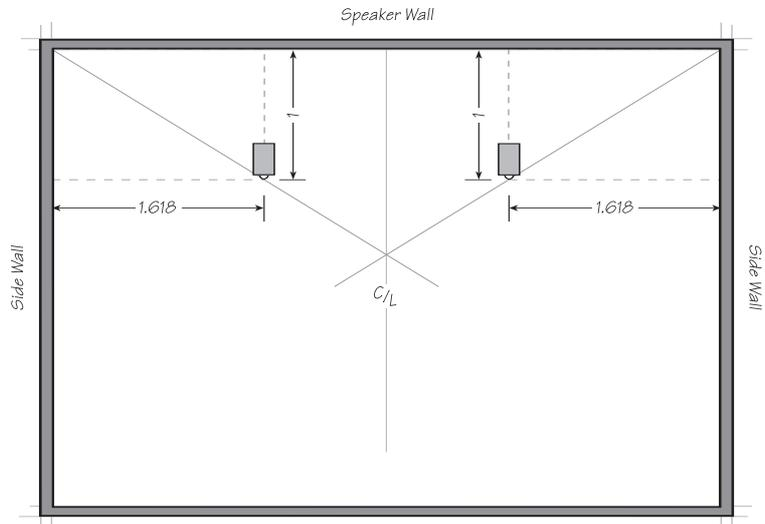
**Golden Rectangles, 1.618 from the side walls x 1 from the rear wall, create diagonal lines for speaker placement in a horizontal room.**
