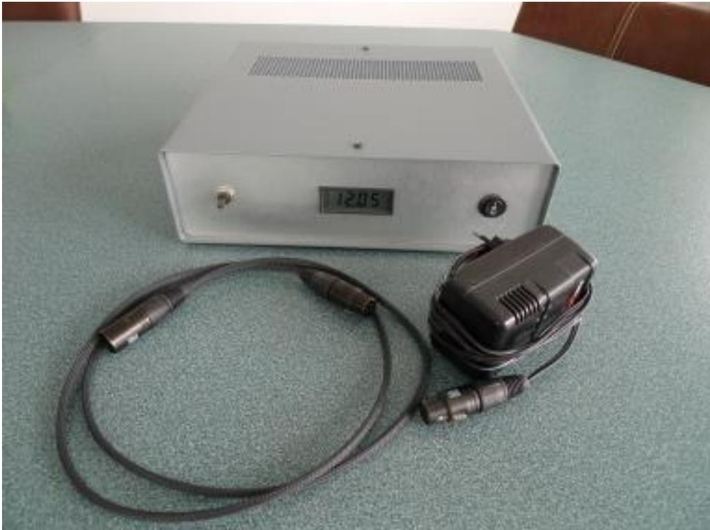
This is one of the kits we used to sell, but any experienced DIY may assemble one. Notice the digital display, a nice and recommended option. We tried many battery types, the dry cell Yuasa works great. Don't go cheap here. 6x 3Ah batteries sum up to 18Ah. We experienced that 18Ah works great. always keep the batteries fully charged at >12,5V when playing. The Yuasa batteries serve about 10 years from our experience.
