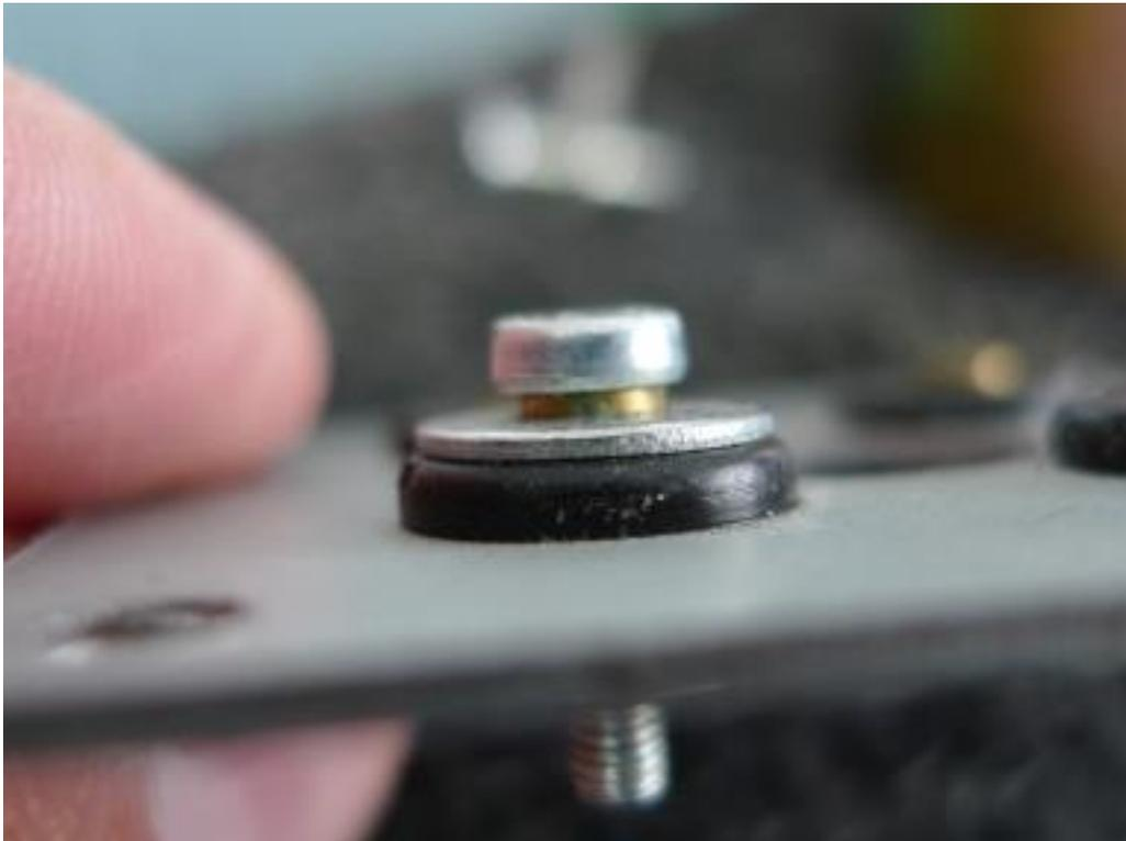
The stock situation. See the brass collar inside the rubber grommet. The assembly may glide up and down, and over time gets play axial and radial.
